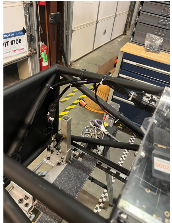
Pictured: Olin Engineering's integrated harness using Alpha Wire's products.
