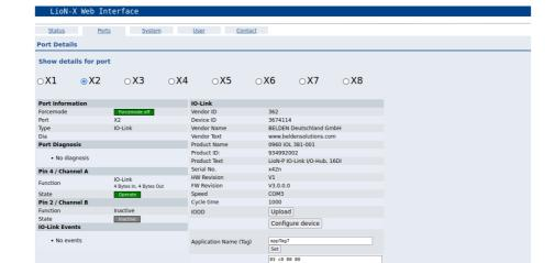
The Port Details Page shows all information about the selected port. In the left column, all port and channel specific information is displayed. If the port is configured as IO-Link and there is an IO-Link Device connected, all IO-Link information for the connected device is displayed in the right column.
