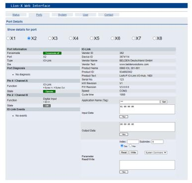
The page shows detailed port information. In the field **Port Diagnosis**, incoming and outgoing diagnostics are displayed as clear text. **Pin 2** and **Pin 4** contain information about the configuration and state of the port. For IO-Link ports, additional information relating to the connected sensor and the process data is displayed.
