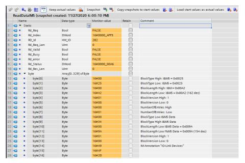
Figure 49: Read example I&M5 on port X1 with connected IOL-Device
