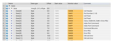
If the resume process has not been finished on the IO-Link Master before the read record is received, a negative PROFINET response will be sent with the code "Resource busy - 0x80C2".
