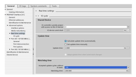
Figure 45: Example of setting up the Watchdog time monitoring in TIA Portal® for using MRP
