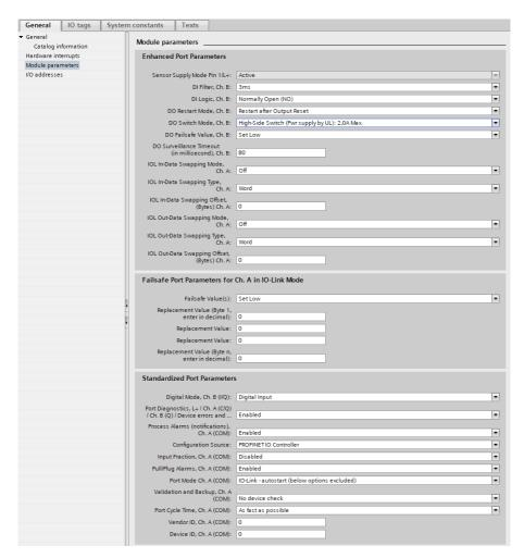
Figure 24: Parameter of the IO-Link channels
