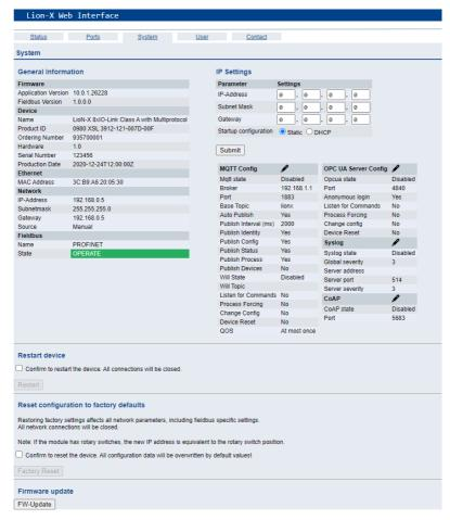
The System page shows the basic information for the module like Firmware version, Device information, Ethernet, Network and Fieldbus information.
