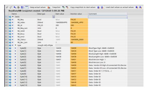
Figure 51: Read example I&M0 on port X1 with connected IOL-Device
