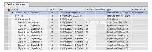
Figure 18: Channels pre-configuration
