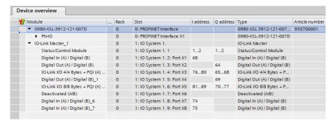
The following options are available for the IO-Link C/Q channel (Ch. A/Pin 4):
