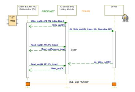
The following table shows the sequence with example data compared to the *FB50001*. The *FB50001* uses the WRREC and RDREC blocks also internally:
