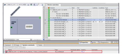
Figure 47: Hardware identifier of the Status/Control Module for RDREC "IO System 1"
