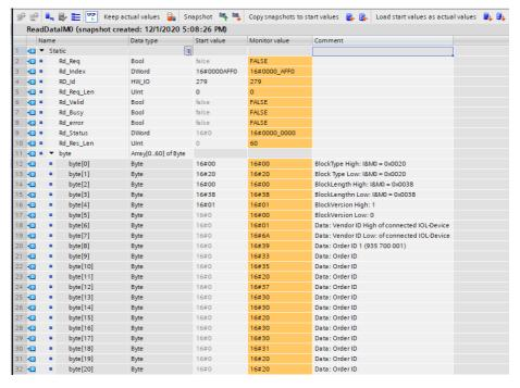
Figure 50: Read example I&M0 of PROFINET IO device
