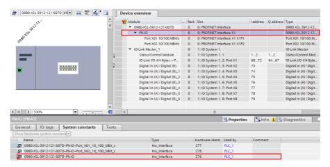
Figure 46: TIA Portal® hardware identifier of PROFINET interface for I&M 0-3 RDREC/WRREC
