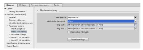
Figure 44: Example of setting up an MRP redundancy client in TIA Portal®
