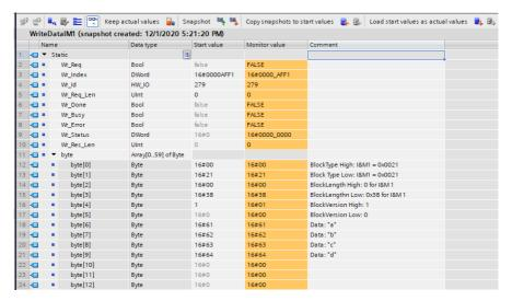
Figure 53: Example of a completed I&M1 write action of a PROFINET IO device
