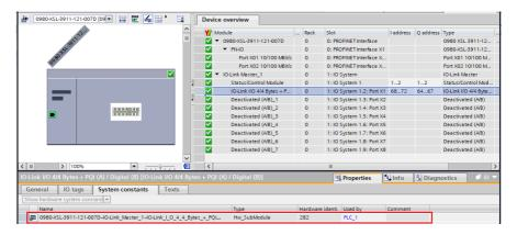
Figure 48: Hardware identifier of the Status/Control module for RDREC "IO System 1.2"
