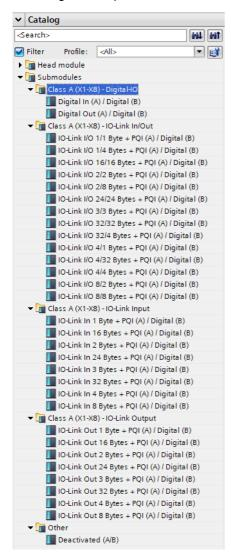
Figure 21: IO-Link channel configuration
