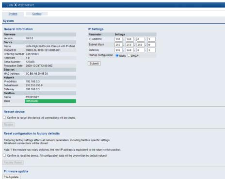
The System page shows the basic information for the module like Firmware version, Device information, Ethernet, Network and Fieldbus information.
