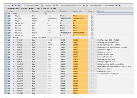
Figure 52: Read example I&M5 on port X1 with connected IOL-Device
