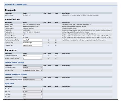
The parameters page "IODD – Device configuration" shows all parameters which are provided by the IODD of the device. That means the parameter set is variable and depends on the connected IO-Link Device.
