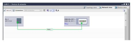
Figure 12: Assign device
