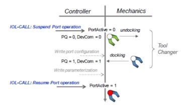
Figure 54: Suspend/Resume Port operation
