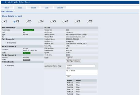
The Port Details Page shows all information about the selected port. In the left column, all port and channel specific information is displayed. If the port is configured as IO-Link and there is an IO-Link Device connected, all IO-Link information for the connected device is displayed in the right column.
