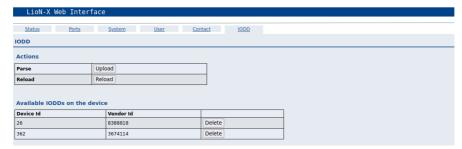
The IODD Management Page can be accessed via the System page displaying all IODDs that are currently stored in the system. All IODDs matching connected devices are marked. On the IODD Management page, you can manually delete any IODD in the system.
