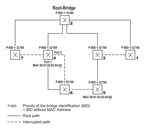
Figure 14: Example of manipulating the tree structure
