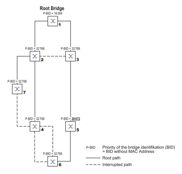
Figure 13: Example of manipulating the root path
