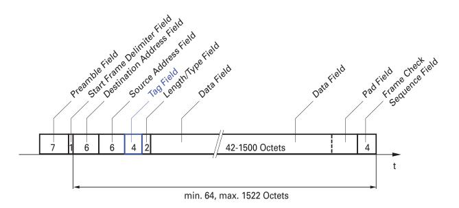
Figure 16: Ethernet data packet with tag
