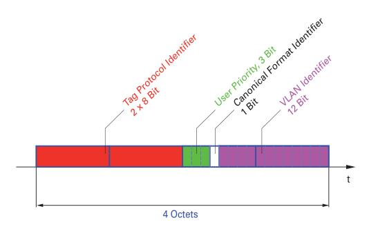
Figure 17: Structure of the VLAN tagging
