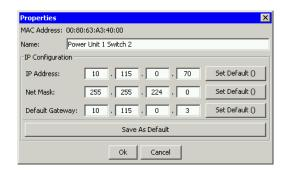
Figure 2: HiDiscovery – IP parameter assignment
