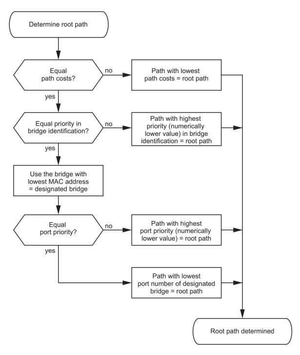
Figure 11: Flow chart for determining the root path
