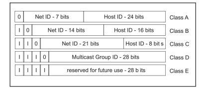
Figure 4: Bit representation of the IP address
