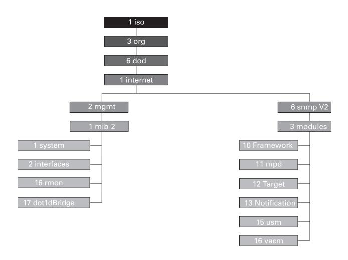
Figure 19: Tree structure of Hirschmann MIB GECKO 4TX
