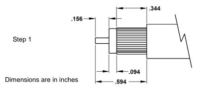
Prepare the cable according to step 1 to achieve the proper braid exposure and center conductor length. Slightly flair the braid away from the dielectric. Twist the foil tightly against the dielectric and verify there are no loose braid strands or foil touching the center conductor.
