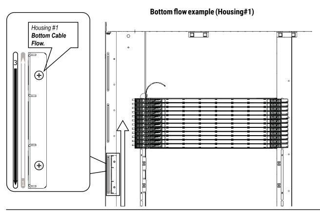
**3**. Determine the angle of the Cable Distribution Manager based on the cable flow.
