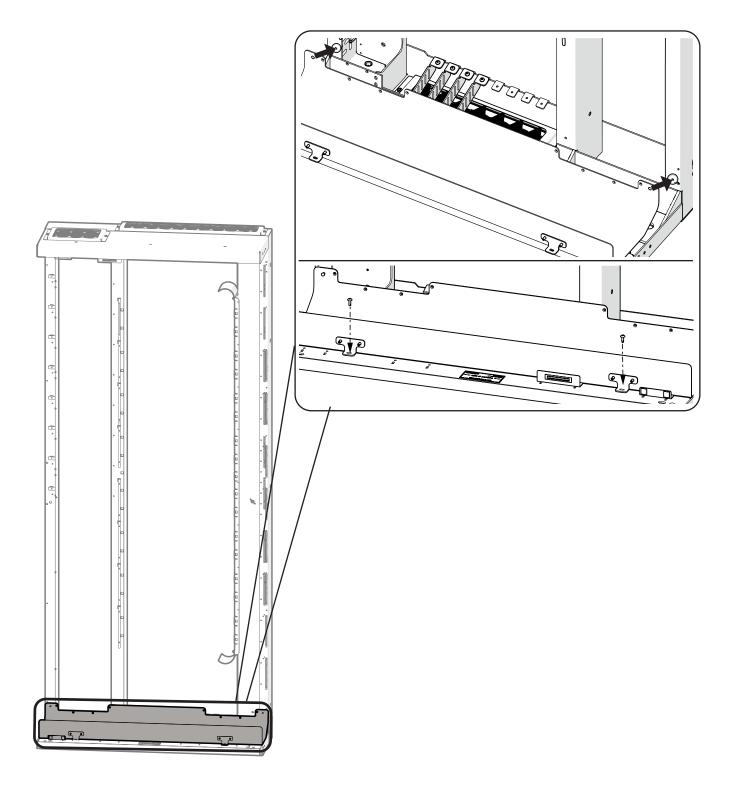
**2.** (If required) continue installing the In-Cabinet Channels to each Cabinets placed as Side-to-Side **NOTE: DCX-HINC-KIT02**<u>x</u> use the same installation procedures shown at the previous page.
