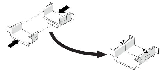
2. Place the Patch Cord Bridge Assembly between two In-Cabinet Channels at the patch cord management area. Intall the plastic screws provided (4 per side) to secure the Patch Cord Bridge from both sides (Front and Rear).
