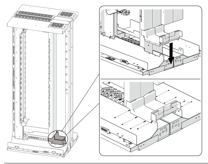
3. (If required) repeat the previous steps shown to continue installing the Patch Cord Bridge Assembly on all Cabinets placed Back-to-Back.
