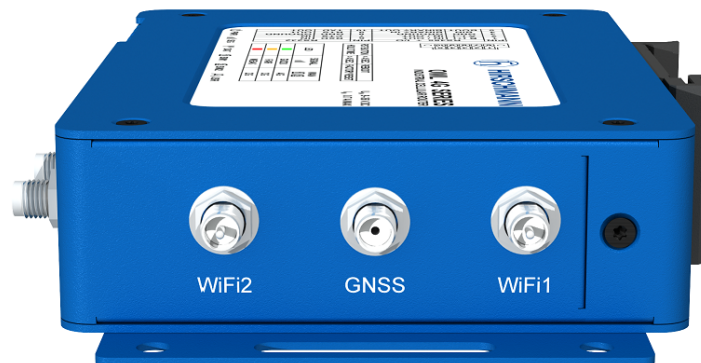
Figure 22: The right panel of the router
