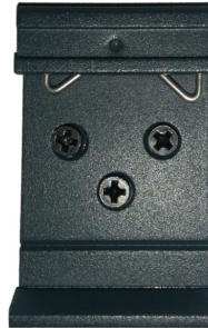
Figure 9: Default position of DIN rail clip
