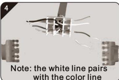
4 Note: the white line pairs with the color line Refer to color and then put the cable into the pressure cap, and cut off the needless cable edge.
