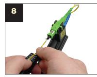
Open the activator tab and insert fiber into the connector. Refer to point D for fiber insertion depth.
