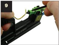
Create a bow and slide the activator tab to the closed position, then bring the boot to the rear of the connector.
