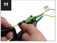
Spread the Kevlar around the threads then gently screw on boot and release bow.
