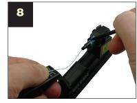
Create and maintain a bow with the fiber, while sliding the activator tab to the closed position (towards boot).
