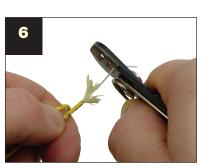
Wrap fiber cable around finger, then strip off buffer to point C\*.
