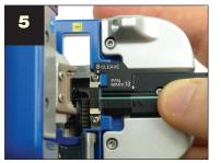
Align the end of the fiber's buffer at 8 mm and cleave.
