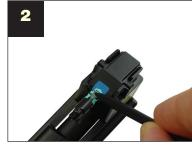
Slide activator tab to the open position (towards ferrule).
