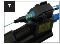
Insert fiber into connector up to the 13 mm buffer mark.
