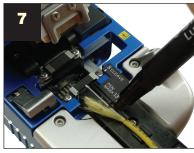
Clean then cleave fiber at  $8_{-0.0}^{+0.5}$  mm.
